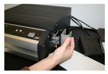
To remove pins, push down on the silver bar and rotate clockwise. Remove pins desired.
