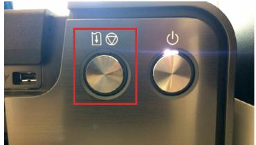
3. When you print a manual feed job, after you hit Print you need to press the "Resume" button on the printer. It is the left button and should be flashing orange when it needs to be pressed.
