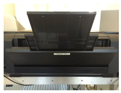
1. The **Manual Feed** is at the back of the printer.
